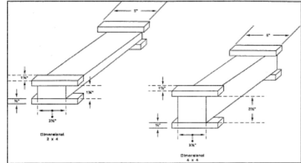
Figure 28-2. Test Fuel Spacer Dimensions.
